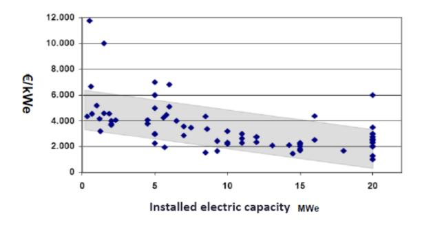
Figure 3.7 Specific investment cost of cogeneration plant for district heating
