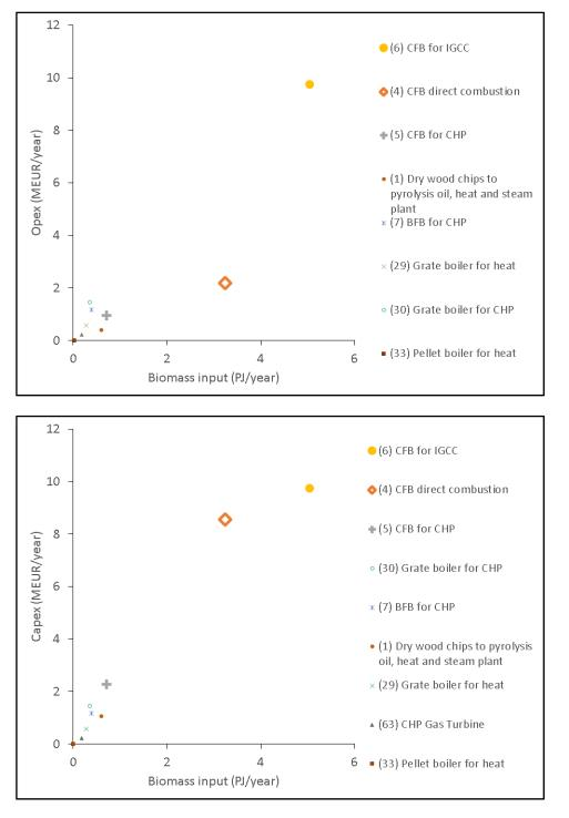
Figure 5. Operation and maintenance (top) and investment (bottom) costs depending of the plant capacity expressed in biomass input for the technologies developed under the WP2.
