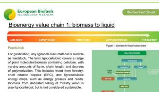
Gasification is a thermochemical process at 800-1300°C run at under-stoichiometric conditions (typically  $\lambda$  = 0.2-0.5). Under these conditions the biomass is fragmented into raw gas consisting of rather simple molecules such as: hydrogen, carbon monoxide, carbon dioxide, water, methane, etc. Solid by-products are: char, ashes and impurities. The gaseous molecules are then chemically resynthesized to biofuels.
